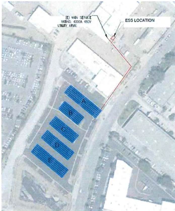
Figure 21: Proposed Solar PV system analyzed by ENGIE over employee and guest parking (Source: ENGIE)
